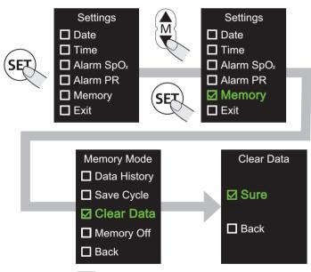
Note: After clearing data, the Micon will show 0 data. Caution: The deleted data could not be restored.
