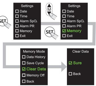
Note: After clearing data, the **M** icon will show 0 data. Caution: The deleted data could not be restored.
