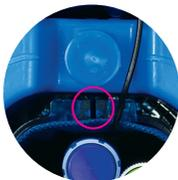
Ensure the thermometer probe peeks out otherwise readings might be inaccurate.
